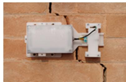
Figura 19. Easy Crack Monitor System®
